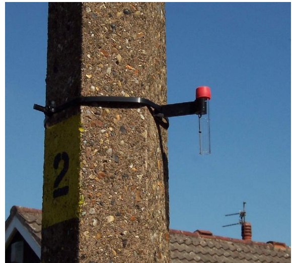
Photograph of nitrogen dioxide diffusion tube used to monitor air quality
